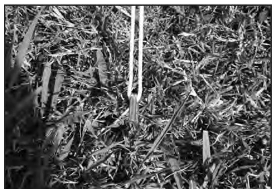
**STEP 21 - Adjust the tension on the guy rope by sliding the clew up or down.**
