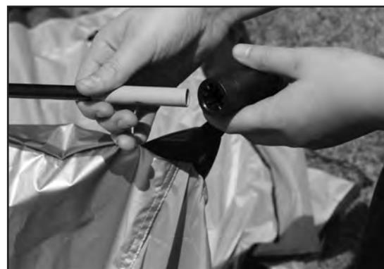
**STEP 3 - Insert pole into the grooved section of the molded corner joint.**
