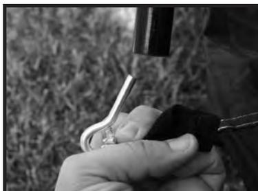
**Step 6 - Insert the pin into the bottom of the leg poles.**
