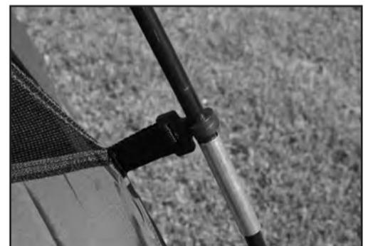
**STEP 6 - Attach speed clips to pole frame.**
