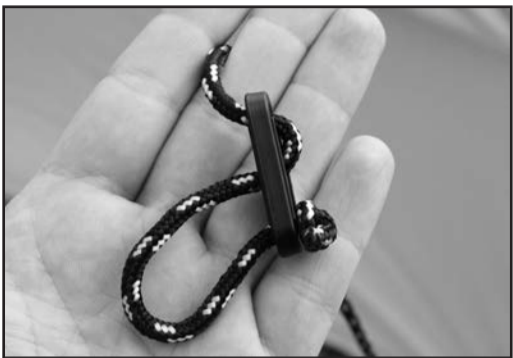
STEP 15 - Loosen the guy rope as shown to wrap around a stake.
