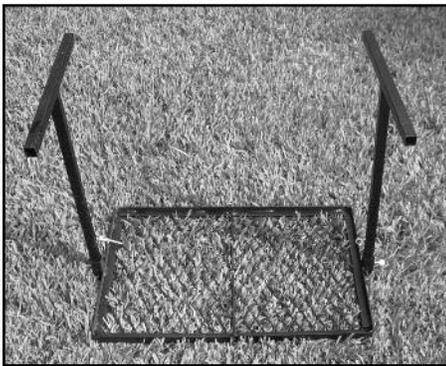
**STEP 1 - Lay grill base upside down and insert the 2 "T" legs into the square leg holders. Secure slightly by turning the screw clamp on each side of the grill.**
