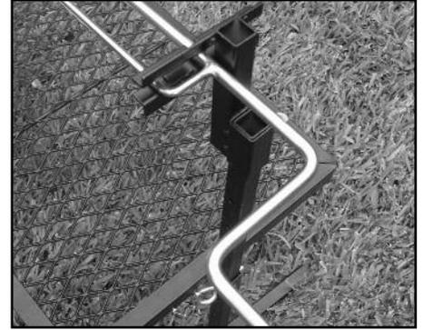
**STEP 12 -** Turning the skewer handle 90° for the second position.
