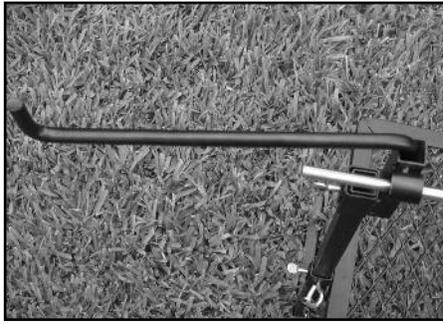
**STEP 8 -** Insert the arm/hot holders into the skewer holder joints.
