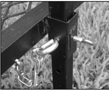
**STEP 4 -** Insert the chained pin into the "T" legs to secure the grill base completely.
