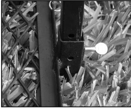
**STEP 2 - Secure slightly by turning the screw clamp on each side of the grill.**
